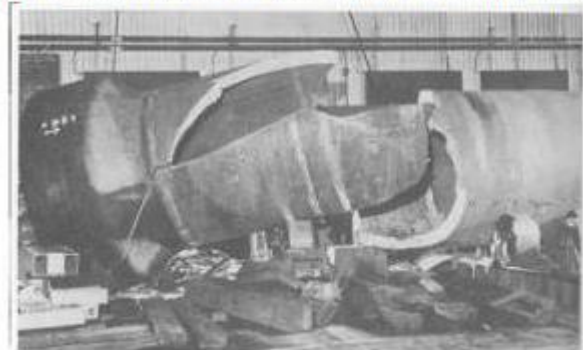
Brittle Fracture of Vessel Shell During Hydrotest
