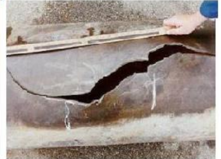
Brittle Fracture of Vessel Shell During Hydrotest
