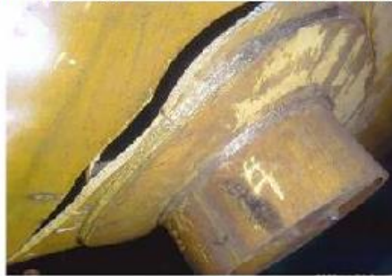
Brittle Fracture of Vessel Shell During Hydrotest
